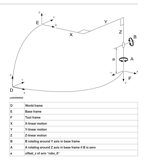
3.2.3.10 Kinematic model XYZC(Z)B(X)A(Z)
